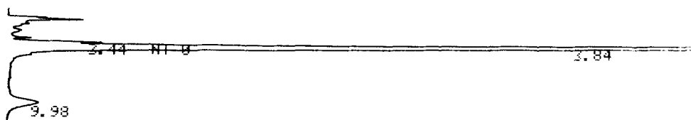
Fig. 4. HPLC analysis of NVPC and lyso NVPC from PLA 2 assay. Solvent: hexane-isopropanol-water 6:8:1.6, 1 ml/min. Fluorescence detection: excitation = 250 nm, emission > 320 nm. Retention times: NVPC, 3.84 min; lyso NVPC, 9.98 min.
